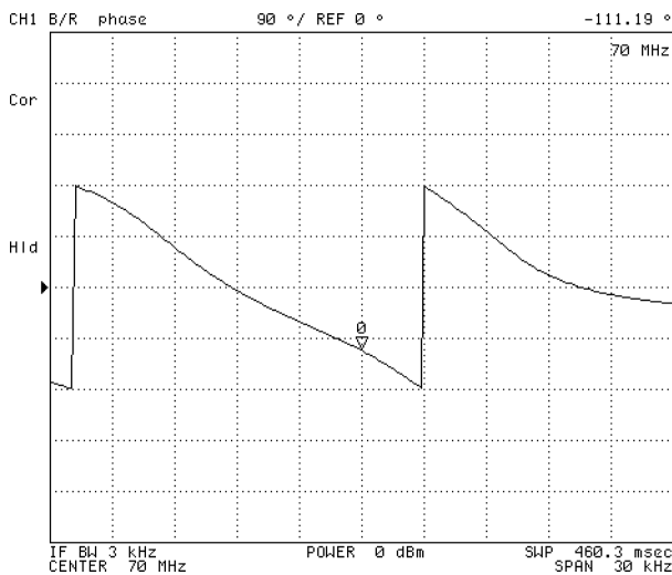
Before Adding the Electrical Length
